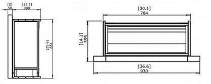
39.50 kg W 930, D 359, H 700 W 930, D 309, H 700 Indoor / outdoor Mild steel, toughened glass Black The 720CV Firebox comes with a stainless steel burner
